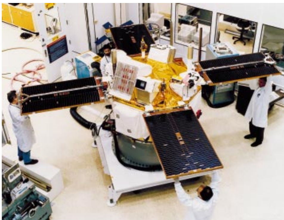
Figure 1. Photograph of the ACE spacecraft during ground testing (solar arrays manually deployed).
