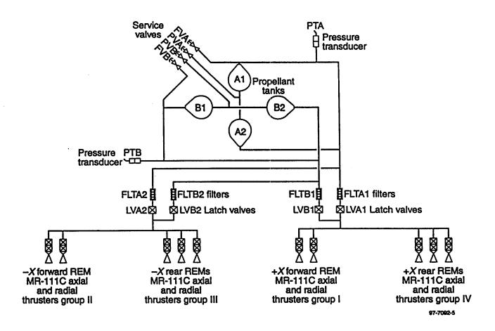
Figure 7.2.6-2: Propusion -- Location and Function of Thrusters
