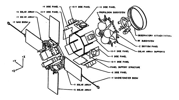
Figure 7.2-1: ACE Spacecraft Exploded View
