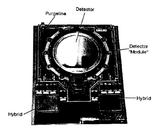
Figure 7.1.2-2: SIS Stack Detector
