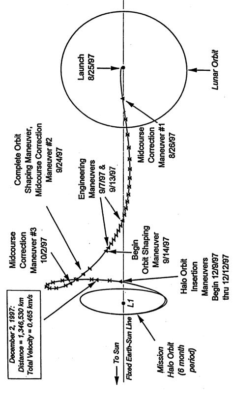
7-day intervals between the Orbit Shaping Maneuver and Halo Orbit Insertion Maneuver Tick marks are at 1-day intervals until the Orbit Shaping Maneuver and
