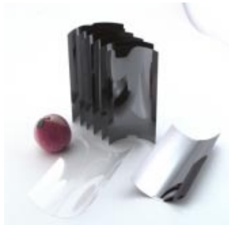
Figure 2. Formed glass mirror shells (300 \mu\text{m} thick) coated with HEFT design W/Si multilayers.
